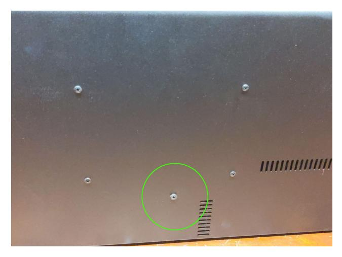
3. Remove the front and top screws on each side panel of the keyboard. The bottom screw on each side is left in place, as that's the hinge the keyboard will open on. Remove the six screws on the back of the keyboard.
