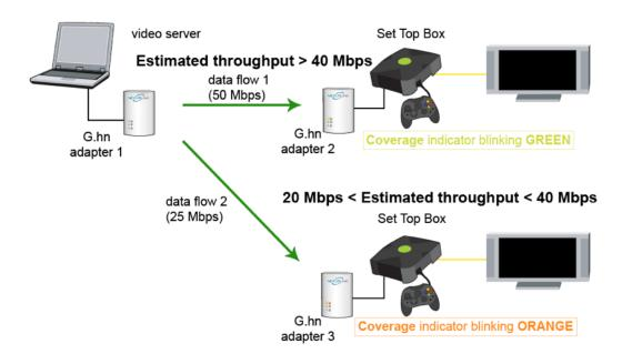
• **CASE 2:** The COVERAGE LED in G.hn adapter 1 will show the estimated level of the PLC link from which it is receiving the most amount of traffic at any given time. For example, if G.hn adapter 1 is receiving traffic at 50Mbps from G.hn adapter 2 and is receiving 25Mbps from G.hn adapter 3, the COVERAGE LED will show the level with reference to the G.hn adapter 2 link, as shown in the following figure.
