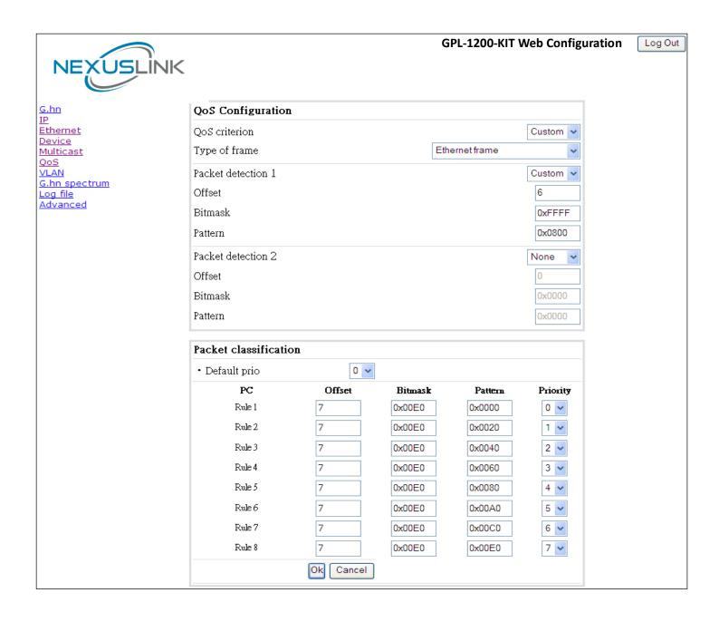
In this case you can reset the factory defaults in the Advanced menu to recall Factory Resets if necessary. If you want to correct this inaccuracy, manually change the values in the Offset boxes to the number 5. Upon clicking the OK button the Offset values will all display 7 respectively.
