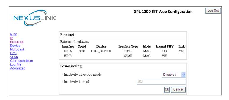
The Ethernet table shows the status & Info of the Ethernet interface; including Interface, Speed, Duplex, Interface Type, Mode, Internal PHY & Link.
