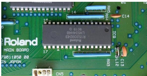
main board flipped over (component side) Note: original 'mkl' IC mounted with lettering upside down and ID hole towards the IC9 name on the board
